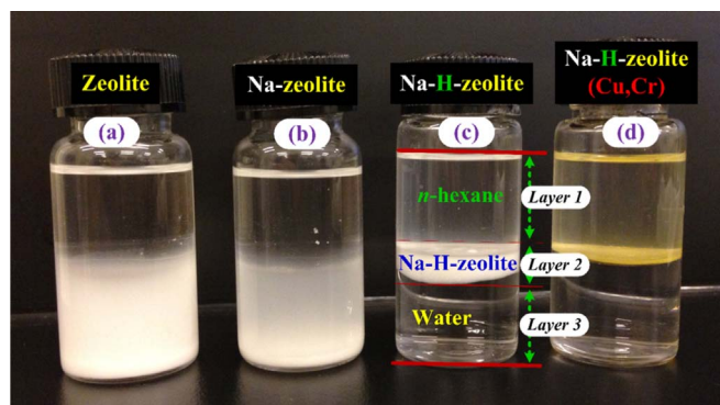
Fig. 1. Distributions of raw adsorbents: (a) pristine zeolite, (b) Na-zeolite, and (c) Na-H-zeolite; and adsorbent after saturated adsorption of \text{Cu}^{2+} and \text{Cr}_2\text{O}_7^{2-} : (d) Na-H-zeolite-(Cu, Cr) in n -hexane/water mixture.
