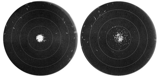
Fig. 1. Examples of image analysis with four concentric circles of 1, 2, 3 and 4 cm diameter placed around the feeding station (left: initial photo, right: day 5). The amount of particles was counted in each ring and used for analysis. (photos: D. Daphi).
