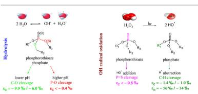
Significant  $^{13}\mbox{C}$  isotope fractionation at lower pH
