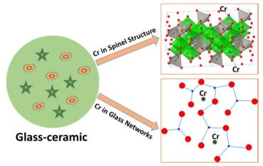
Schematic illustration of chromium incorporating in the glass-ceramic matrix. Most chromium contents are incorporated into spinel structure where the residual chromium are resided in the glass networks.
