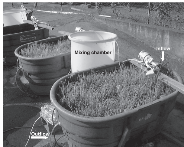
Fig. 1 – Mesocosm setup with pesticide mixing chamber, piston pump for pesticide delivery, inflow tubing, and outflow tubing for collection of sample.
