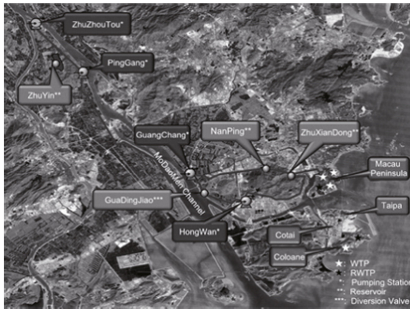
Fig. 1 – Raw water supply system of Macau.
