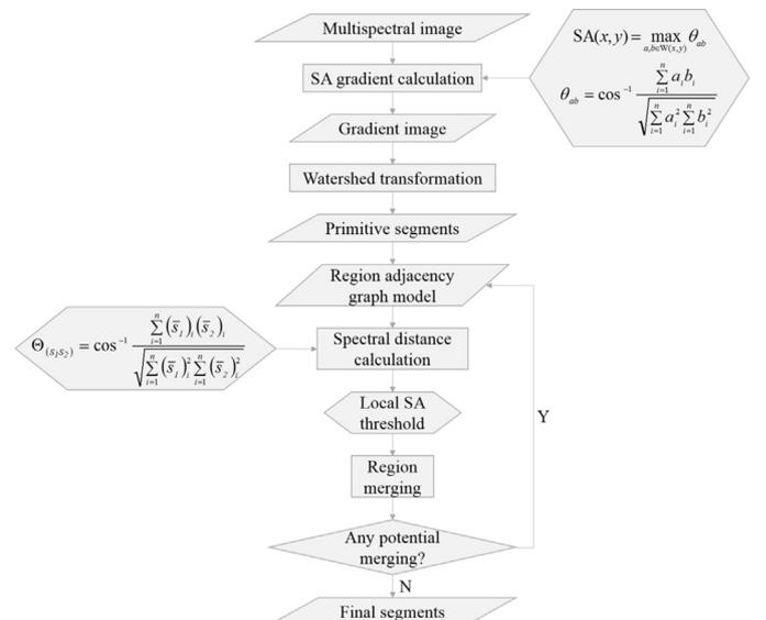
Fig. 1. Hybrid method for multi-scale segmentation using spectral angle thresholds for local region merging.
