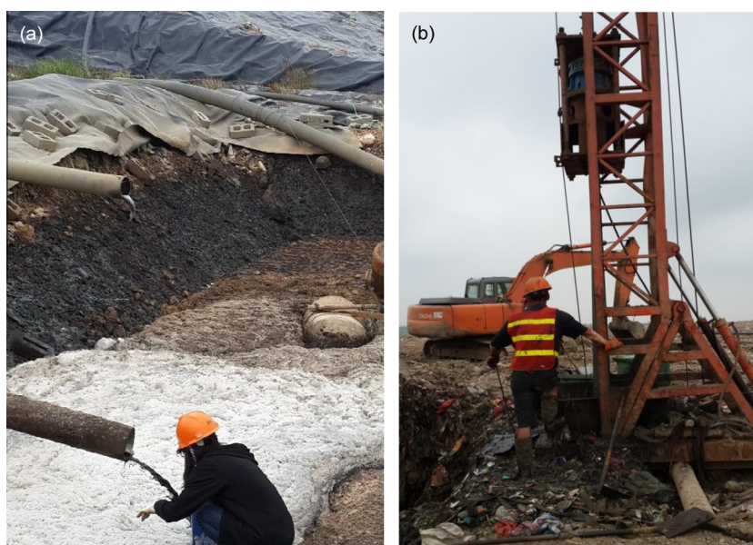
Fig. 1. Sampling process at Laogang Landfill: (a) leachate sampling; (b) MSW sampling.
