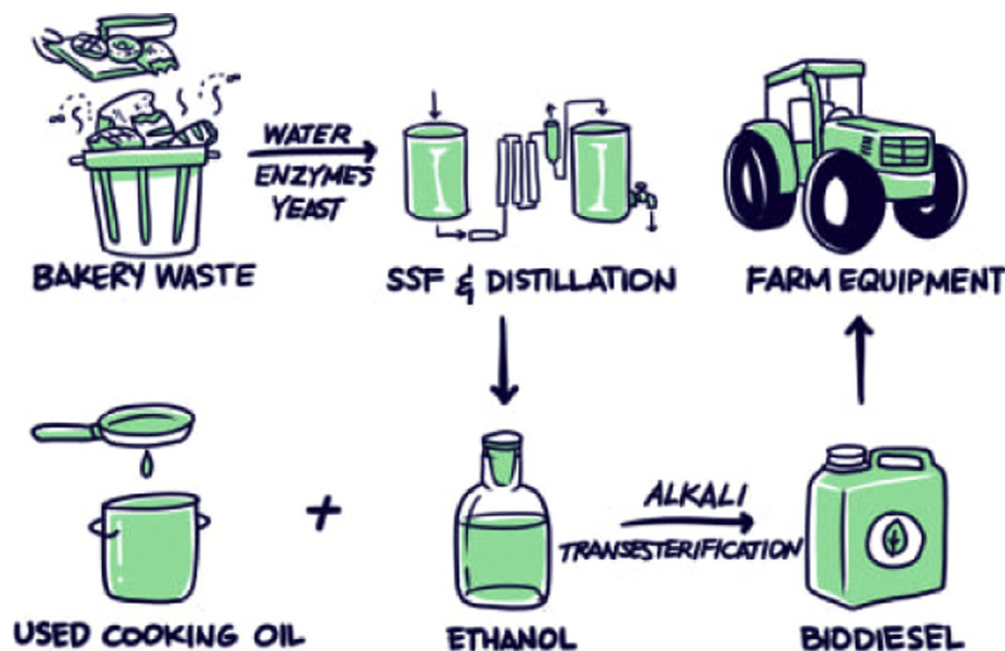
Fig. 1. Concept picture showing how pie waste could be converted into biodiesel. Ethanol produced from pie waste could be processed with used cooking oil from restaurants in the presence of alkali using trans-esterification process to produce bio-diesel that could be used in farm equipment's.
