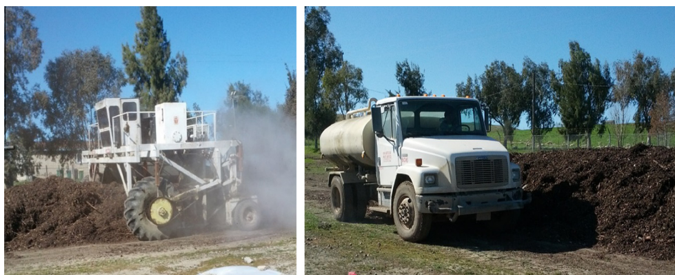
Fig. 1. Photograph of scarab turning the experimental windrow pile (left) and the water truck spraying the experimental windrow pile (right).
