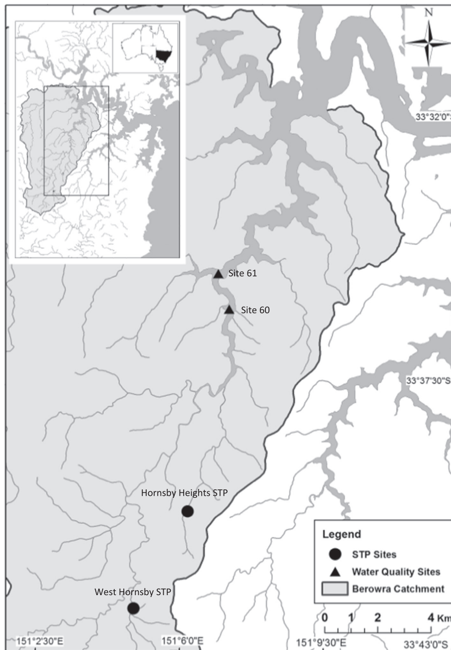
Fig. 1. Map of Berowra Creek estuary located within the Lower Hawkesbury Nepean estuary in New South Wales, Australia. Large map shows locations of two sewage treatment plants Hornsby Heights and West Hornsby (dark circles) and sampling sites 60 and 61 (dark triangles) downstream of the facilities.
