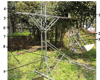
1. Designed system; 2 and 6. Cross beam; 3 and 5. Slide bars; 4. Halyard; 7. Straight beam; 8. Guide rails; 9. Capstan
