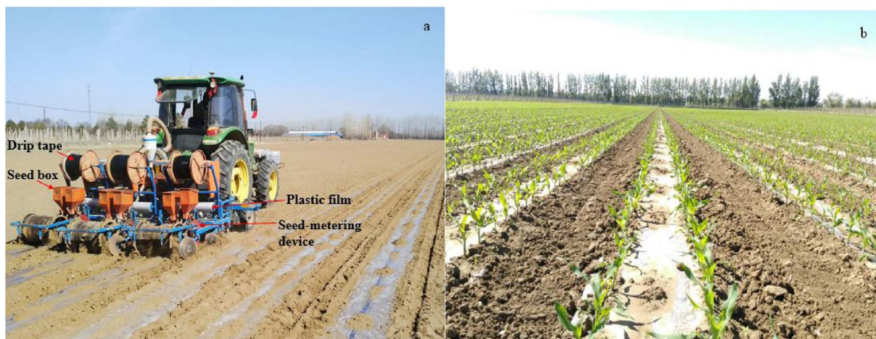
Fig. 1. Joint planter applying drip tape, plastic film, punch holes and sowing.
