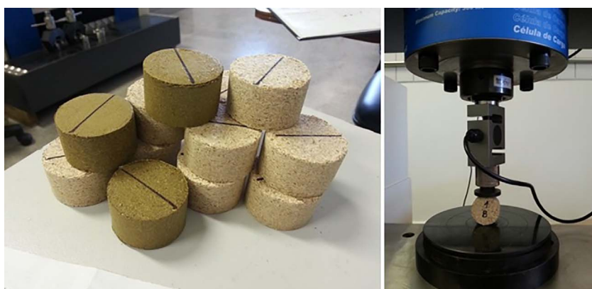
Fig. 1. Briquettes samples and diametrical compression test.
