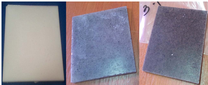
Fig. 1. Epoxy composite, 1% and 3% nano OPEFB/epoxy nanocomposites.
