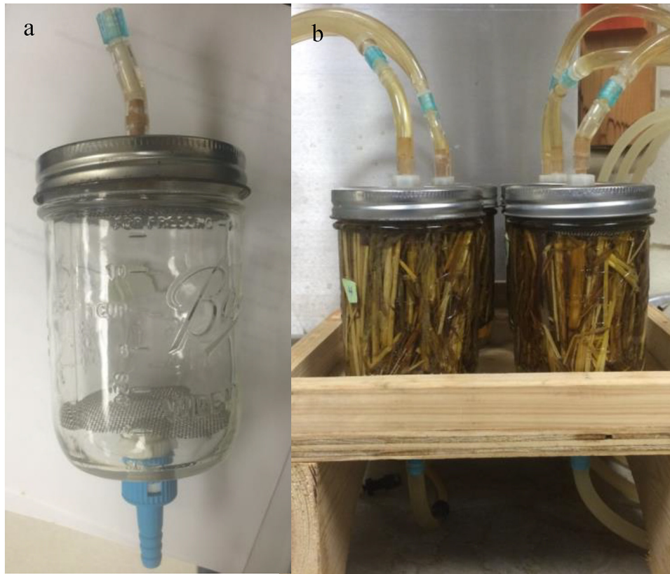
Fig. 1. a) Vessel used for up-flow treatment showing in-flow port on the bottom of the vessel and exit port on the top. b) Stand showing six vessels in use simultaneously during high solids recirculating \text{Ca}(\text{OH})_2 pretreatment.
