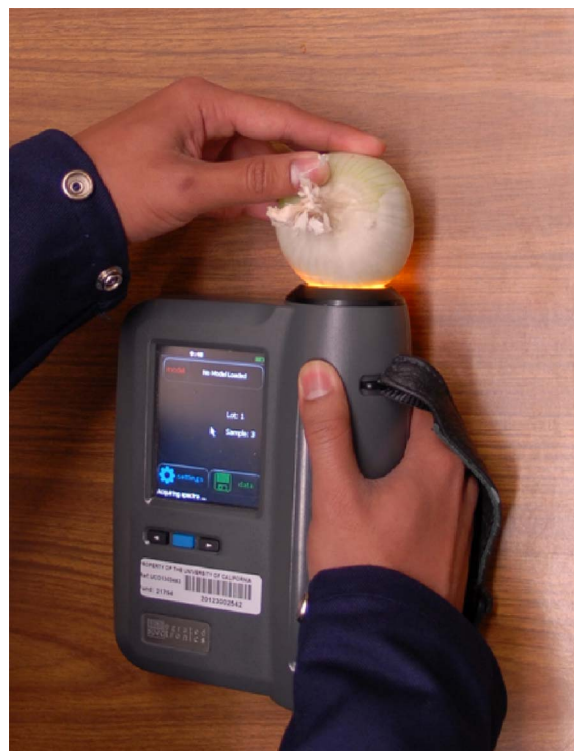
Fig. 1. Handheld visible-NIR spectrometer being used to measure the interactance spectrum of sample.
