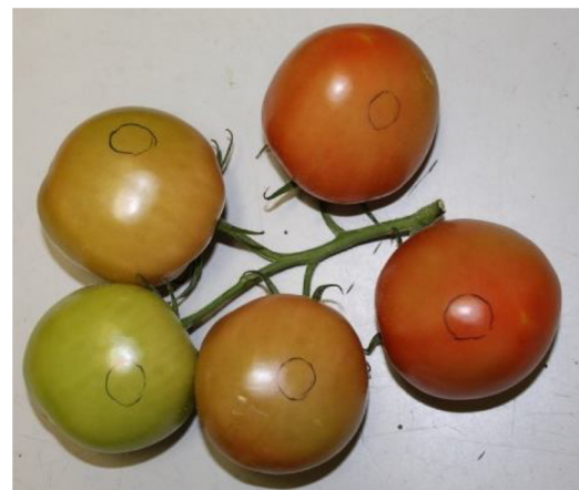
Fig. 2. Tomato vine of the cultivar Merlice with the marked circles at the bottom of the tomatoes where the calibrated spectrophotometer measurements were performed.
