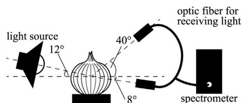
Fig. 1. Schematic diagram of spectral measurement.
