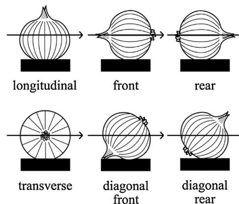
Fig. 2. Six positions during spectral measurement. Arrows indicate the traveling direction of irradiating light, i.e., the optical axis of the system.
