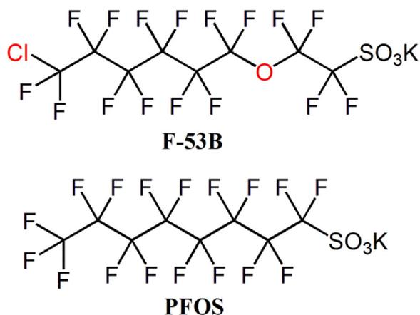
**Fig. 1.** The molecular structural differences between F-53B and PFOS, red color indicates atoms different from PFOS. (The reader is referred to the web version of this article to view the figure in color.)
