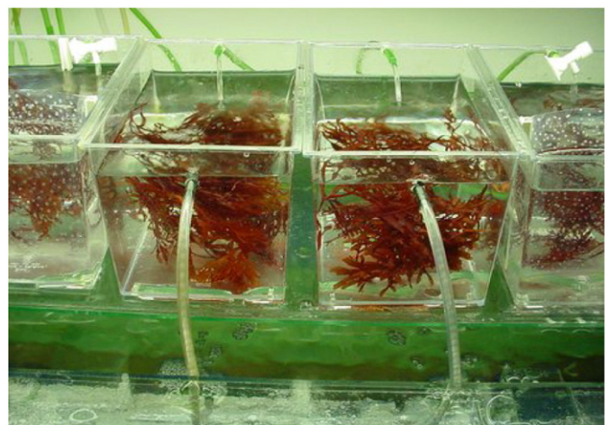
Fig. 1. Rectangular transparent plastic aquaria (12 × 18 × 11 cm, volume = 2 l) used as experimental units, EU.
