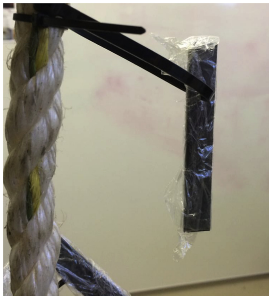
Fig. 1. Carbon steel coupon attached to the fiber rope prior to exposure, with protective plastic wrap.
