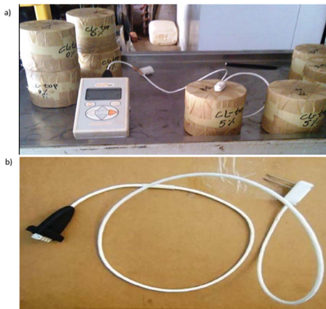
Fig. 1. Measurement of thermal properties in laboratory: (a) Set up of the measurement process (b) the dual SH-1 sensor for measuring thermal properties.
