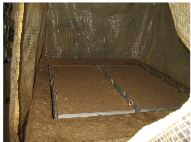
Fig. 1. The rain simulator soil boxes and the buffer area in their vicinity. Each plot is 116.5 × 55 cm.
