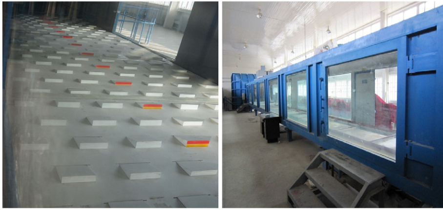
Fig. 1. The wind tunnel with roughness.
