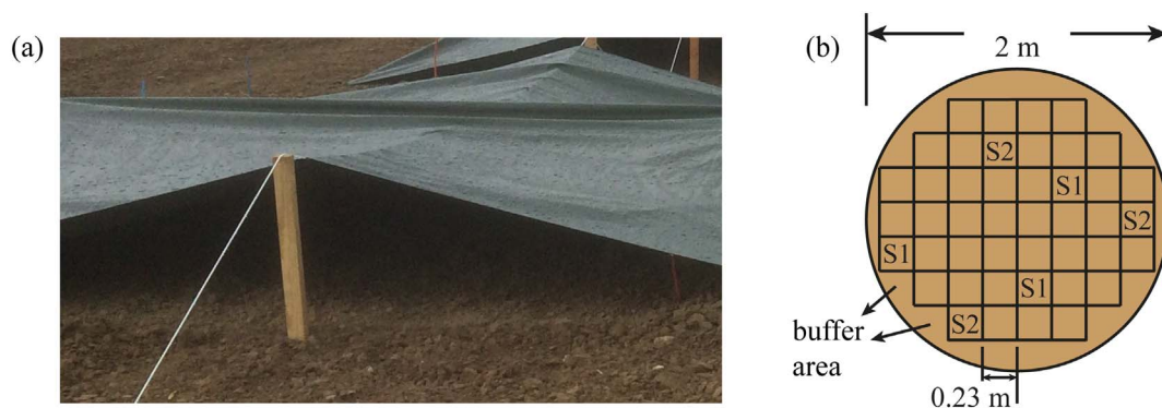
Fig. 1. (a) Waterproof plastic cover protecting the surface of an experimental plot against natural rainfall and allowing ventilation during dry periods. (b) Experimental plot layout with sampling grid. S1 and S2 represent examples of randomly assigned grid cells from which replicate samples were taken at the first two out of 13 consecutive samplings.
