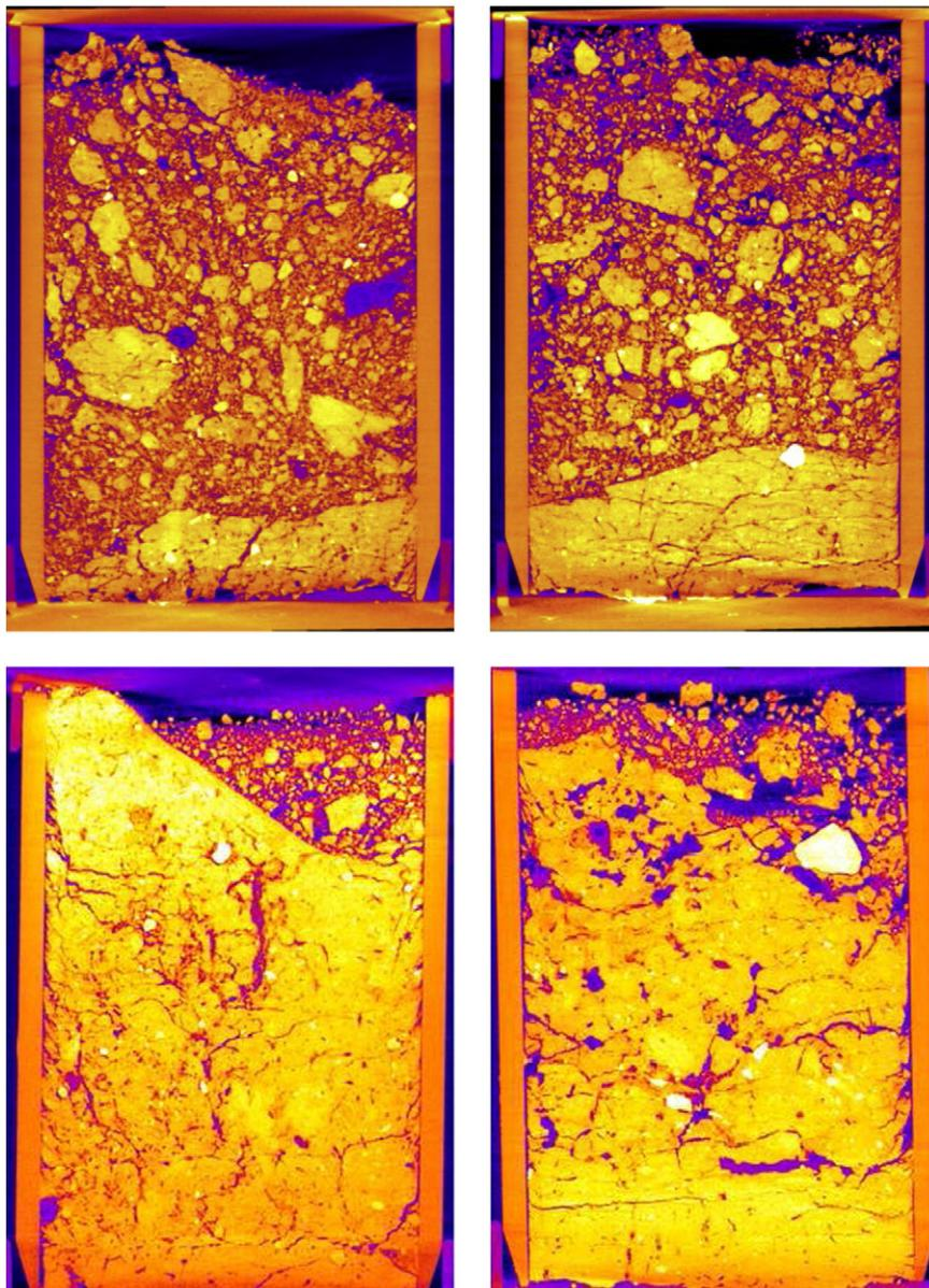
**Fig. 1.** Four example 2D images of vertical slices through samples (inner diameter 6.7 cm) taken at Offer, illustrating the contrasting structures in the harrowed and ploughed layers. The two uppermost images are samples taken from the soil surface, the two beneath are from 10 to 20 cm depth.
