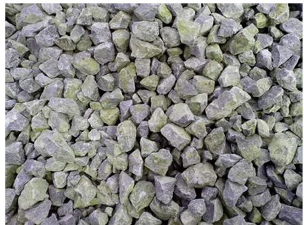
Fig. 1. The crushed stone gravel used in experiment.
