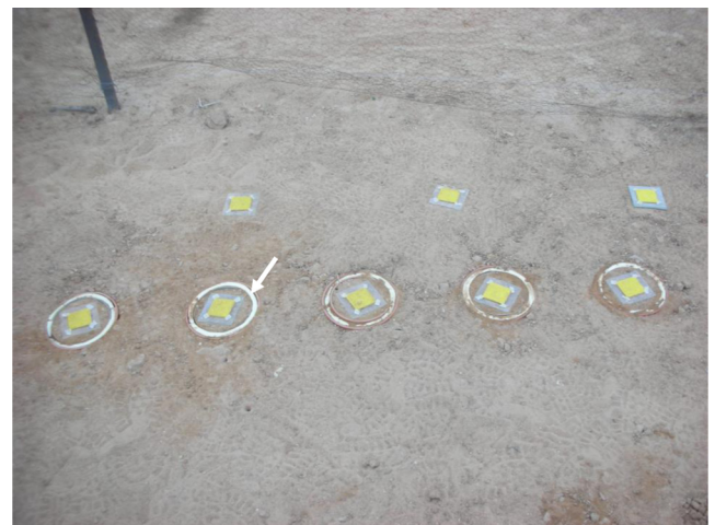
Fig. 1. Micro-lysimeters (bottom) and glass plates serving as control (top) in the field. Arrow points at the 1.5 cm-wide and 2.0 cm-thick polyurethane ring inserted in between the inner and the outer pipe aiming to reduce heat loss through the air gap.
