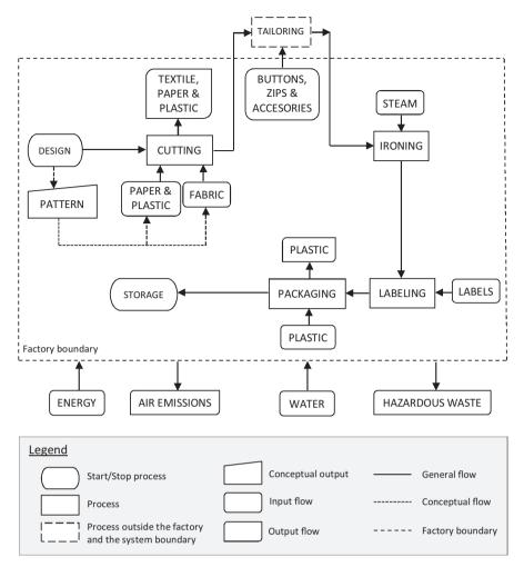
Fig. 1. Dressmaking factory process flowsheet.
