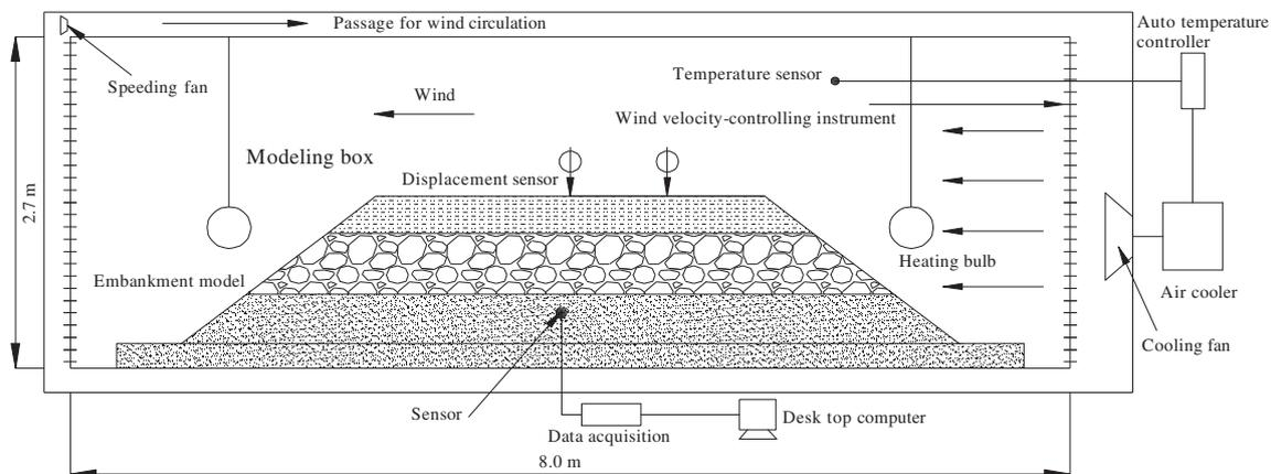
Fig. 1. A schematic diagram of the experimental equipment.
