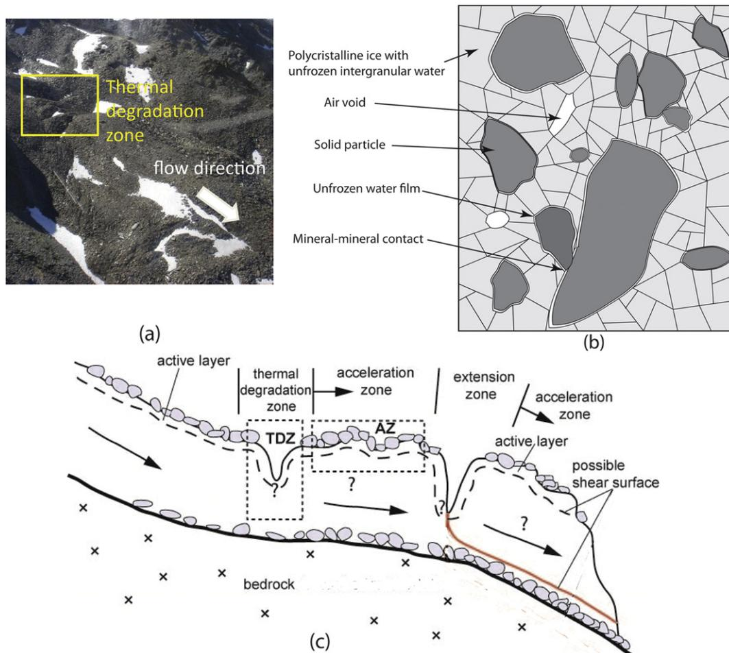
**Fig. 1.** a) aerial view of the Furggwanghorn rock glacier, Turtmanntal, Valais, Switzerland. (Photograph, Sarah Springman), b) Two-dimensional schematic of the structure of frozen soils (after Ting et al., 1983), c) Schematic cross section through a degrading rock glacier (after Springman et al., 2011).
