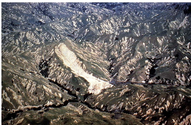
Fig. 1. A large, multiple-occurrence regional landslide event resulting from Cyclone Bola rainfall of 300–900 mm in 72 h, affecting an area of over 8300 km 2 , March 1988, East Coast, North Island, New Zealand (photo: Noel Trustrum).
