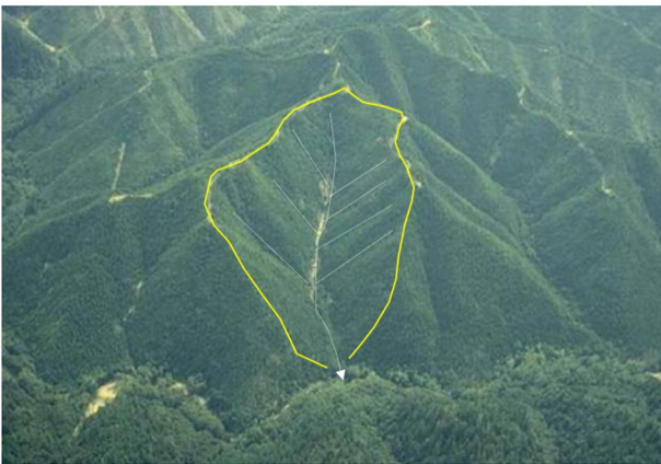
Fig. 1. Debris flow catchments. This oblique aerial photo (photo by J. Roering) shows characteristic debris-flow-dominated catchments in the Oregon Coast Range. Yellow outline delineates catchment boundaries while the dotted white lines illustrate the primary debris flow tracks that terminate in unchanneled valleys just below the ridgetops.
