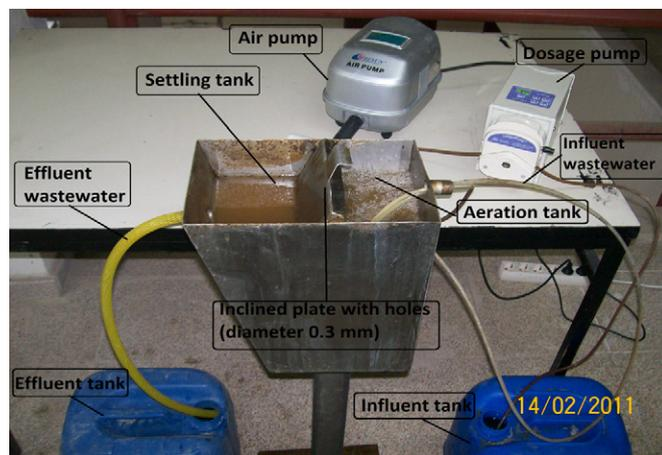
Fig. 1. Configuration of aerobic activated sludge reactor (AASR) system.
