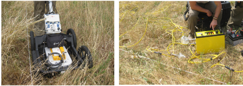
Fig. 1. (Left) MALÁ GPR PRO-Ex with a 500 MHz shielded antenna mounted on a cart at the site. (Right) AGI SuperSting R8 ERT resistivimeter with cables and stainless steel electrodes.
