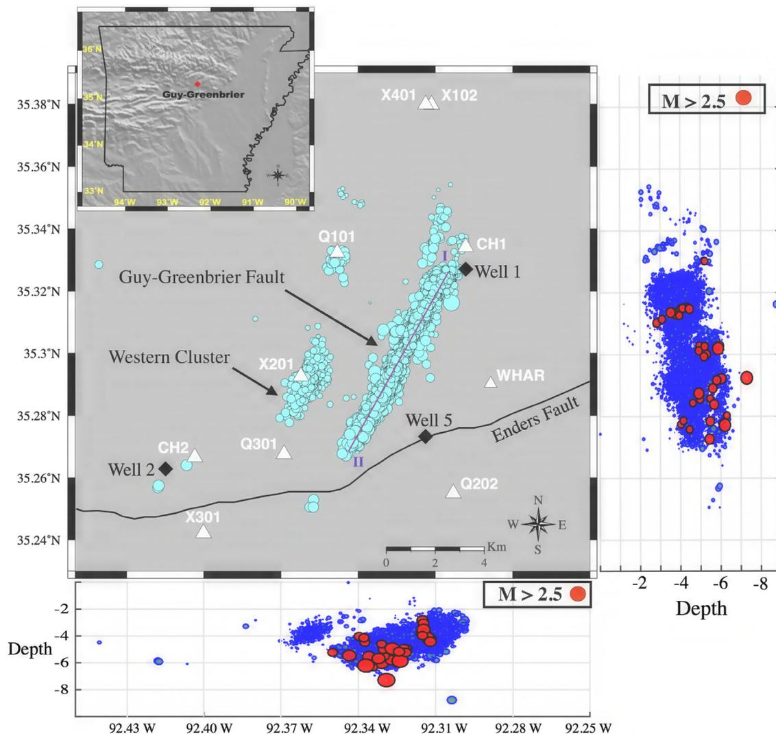
Fig. 1. Epicentral and cross-sectional distributions of seismicity in the study area (between 7 July and 20 October 2010). Marker sizes are scaled to event sizes. Seismic stations are shown by white triangles and black diamonds are disposal wells. The Enders fault is shown by a solid black line.
