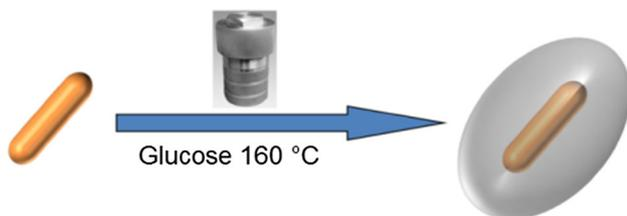
**Fig. 1** (Color online) Schematic illustration of AuNR@Carbon nanocapsule fabrication
