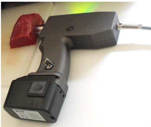
Fig. 1. Hand held Raman spectroscopy sensor head measuring a fresh intact lamb SM, with the epimysium removed.
