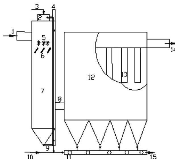
**Fig. 1.** Schematic diagram of the experimental setup: (1) Flue gas Inlet; (2) Humidification Unit; (3) Humidification Water; (4) Bucket Elevator; (5) Internal Mechanical Raking; (6) Internal Diversion Plate; (7) DPT Desulfurization Reactor; (8) Middle Flue gas Channel; (9) Tower Bottom Conveyor Scraper; (10) New Desulfurization reagent; (11) Circulating Ash Transport System; (12) Bag-type Dust Collector; (13) Bag; (14) Flue gas Outlet; (15) Discharge Ash.
