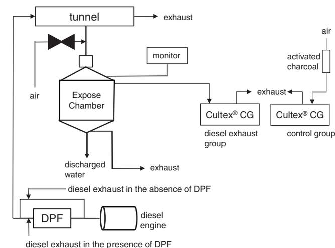
Fig. 1. Schematic of the configuration of the air–liquid interface exposure system.
