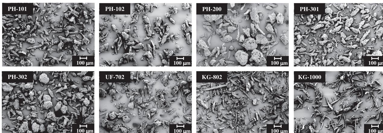
Fig. 1. SEM images of the different types of MCC particles.
