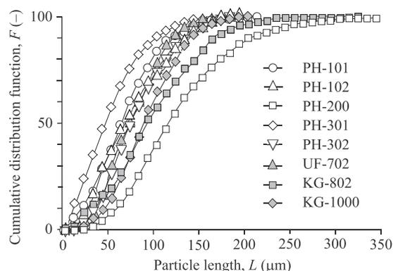
Fig. 2. Cumulative distribution functions ( $F$ ), of the major axis lengths ( $L$ ), of the MCC particles.
