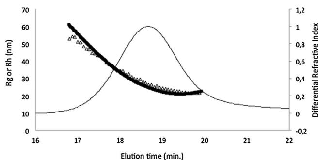
Fig. 1. Elution chromatogram obtained from SEC-MALLS of liposomes composed by DMPC and DMPG (65:35, mol:mol) and obtained after 9 sonication cycles. dRI signal (—),  $R_g$  (■) and  $R_h$  (△) are plotted as a function of the elution volume.
