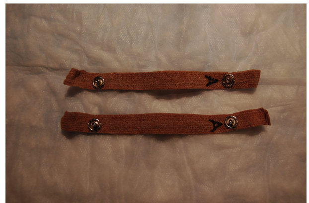
Fig. 1. RespiRod bands. The minimum total stroke volume that these bands can detect is 3 cc at a respiratory frequency of 120 breaths per minute, with a minimum positive end-expiratory pressure of 3 cm H 2 O.
