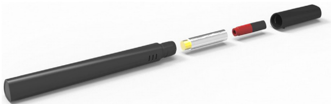
Fig. 1. Schematic of the external appearance and parts of the tested EVP. From left to right, pieces are: the housing, which contains the battery and has a LED indicator on the side, the atomiser, the capsule containing the e-liquid and the mouthpiece.
