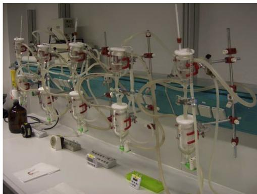
**Fig. 1.** Ex-vivo perfusion equipment constructed according to the design devised by Fisher and Parson (1949), modified from Schumann et al. (1986), (left, Perfusate = perfusate, Resorbat = absorbate; Fig. from Richter and Strugala, 1985) and the laboratory set-up of five sets of perfusion equipment forming an ex-vivo perfusion battery (right).
