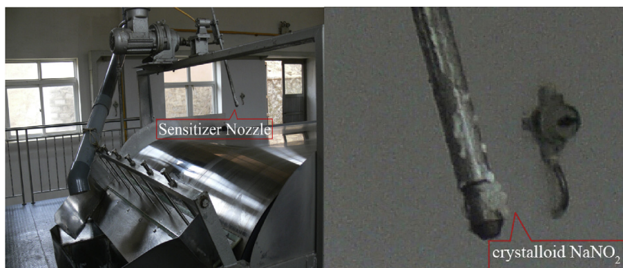
Fig. 1. Scene picture in sensitization process with a close-up of the sensitizer sprayer nozzle.
