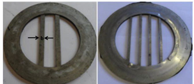
Fig. 1. Turbulence generation obstacles: two and four flat-bar obstacles of 20% blockage each.
