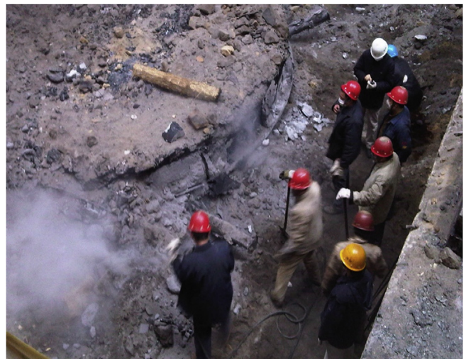
Fig. 4. Cake-like residues inside the molding pit after explosion.
