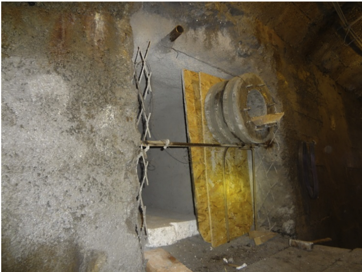
Fig. 1. An entrance of the supply borehole OI, trespassing brick and concrete casing surrounding the underground reactor, responsible for media supply to the gasification process.
